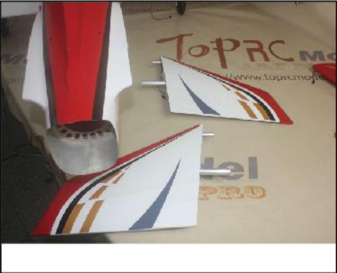
42.Lock the stabilizers to the fuselage by screws from the top of the tail fuselage.
