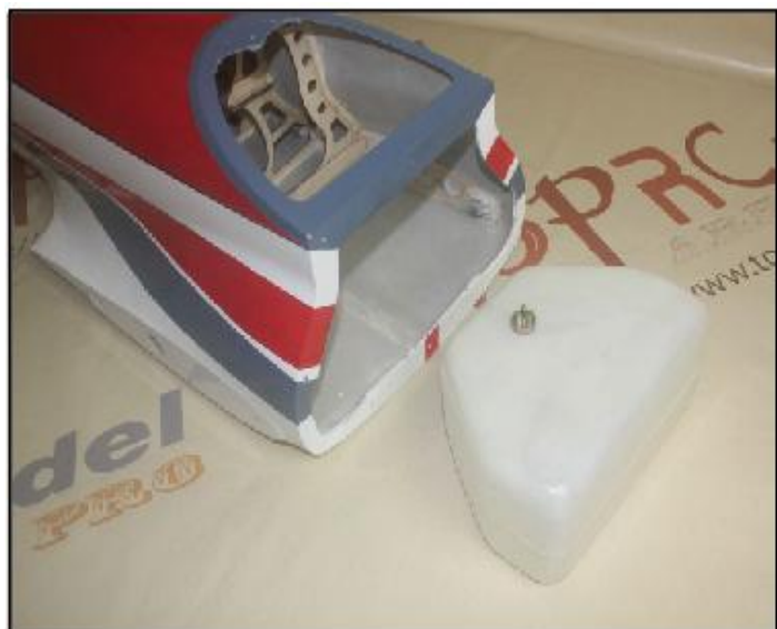
32.Put the fuel tank into the fuselage.
