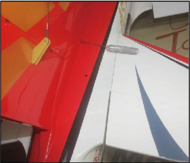
45.Assemble the vertical fin to the fuselage, lock it with screw from the hole in the tail fuselage as picture.
