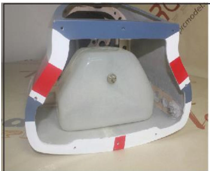
32.Put the fuel tank into the fuselage.
