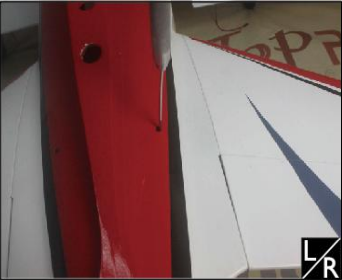
42.Lock the stabilizers to the fuselage by screws from the top of the tail fuselage.
