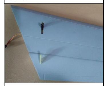
18. Connect the arm of servo to the horn with push rod.
