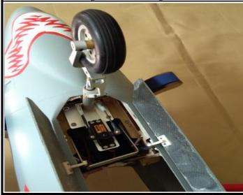
42. Connect the clevis to the hatch hinge with screws and nuts.
