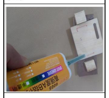
4. Epoxy the wood block to the servo tray tightly.
