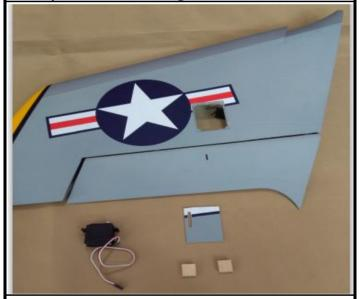
2. Put the wood block to appropriate position base on the servo tray, mark out with red.
