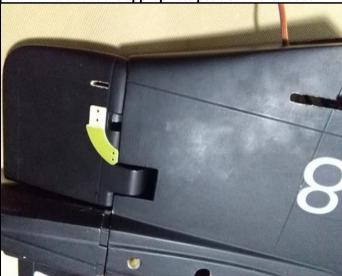
30.Put masking tape around the slot to keep the plane body clean after work done.
