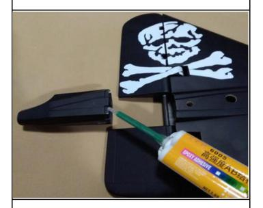
23. Assemble the tail cone to the vertical fine tightly.
