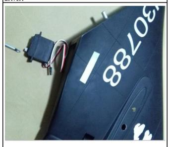
28. The sketch map after the servo of rudder assembly.
