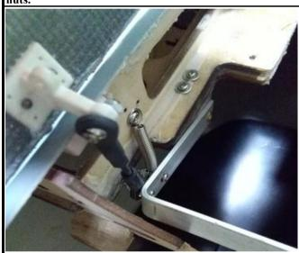
44. The servo parts for the air brake.
