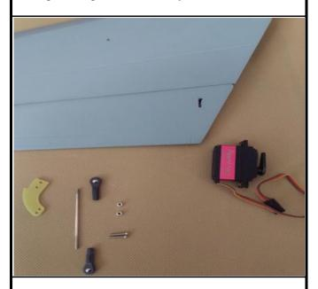
15.Measure the deepth and mark out where the servo would location.
