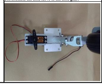
39. Bending the push rod to a propriate angle and assemble them to the retainers .
