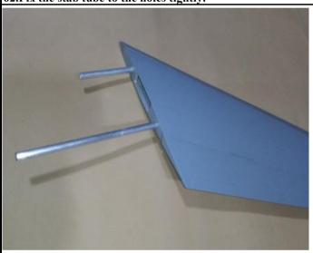
63. Assemble the stab to the fuselage and lock it to the fuselage with screws.
