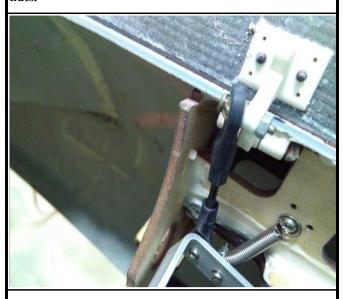
43. Connect the clevis to the hatch hinge with screws and nuts.
