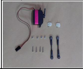
45. Assemble the nylon horn to the air brake inner side, assemble the air brake servo to appropriate position in the fuselage, connect the horn to the servo arm with push rod.
