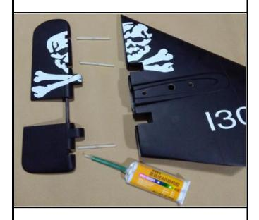
20. Apply instand type AB glue to the slots in vertical fin.
