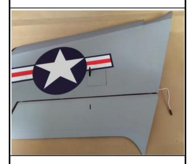
7. Drag the servo line out of the wing.
