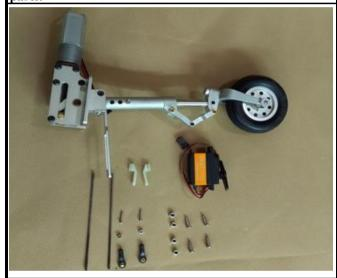
38. Assemble the nose servo to the nose gear.
