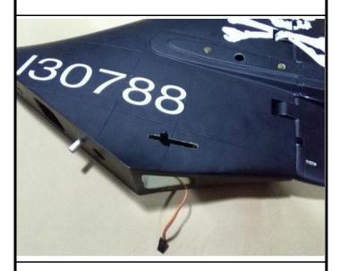
29. Trim a slot at the appropriate position in the rudder.
