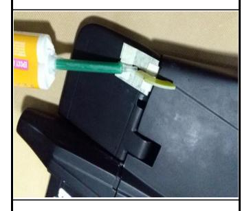
32.Remove the masking tape after the glue dried.
