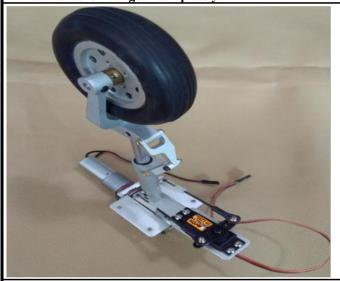
41. Assemble the nose gear to the fuselage with screws.
