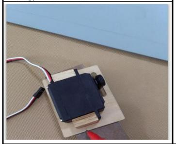
3. Epoxy the wood block to the servo tray base on the mark line.
